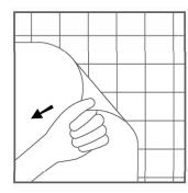
step 6 After approved setting time you may remove excess thinset from grout joints with a razor knife if necessary. Peel the face tape, starting at the corner if applicable. Clean any tape residue with a damp sponge.
